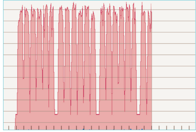
FIG 3 – processor activity trace using multi-threaded compositing and rendering, in combination with Harlequin Parallel Pages is 1.3 times faster.
