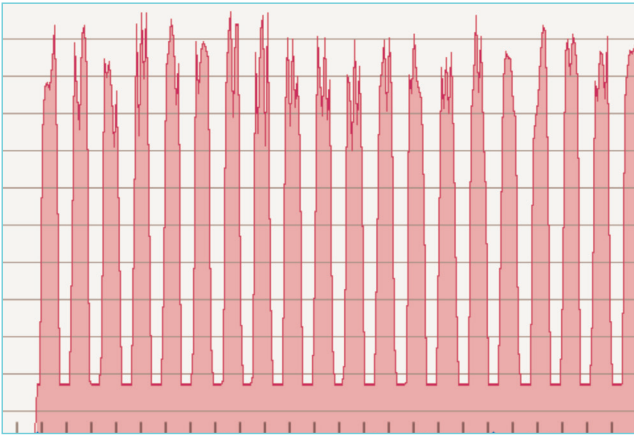
FIG 2 – processor activity trace using multi-threaded compositing and rendering, but not Harlequin Parallel Pages™.
